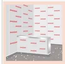
Fabricate an 18 gauge stainless steel 'U' shape capping with welded corners cleaned off flush. Make sure all edge are blunt and safe for cleaning.
