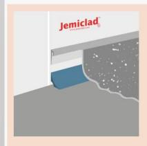
If the Jemiclad is installed to the floor, sheet vinyl can be installed on top. The flooring contractor is to specify cove base, capping trim and adhesive to be used.
