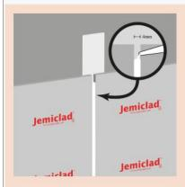
Install Jemiclad onto Jemifix double-sided tape, keeping the joint 4mm apart using a 4mm spacer.
