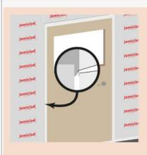
Install Jemiclad 2–4mm from the door detail to allow Jemiclad finish sealant to toe into the gap and become structural.
